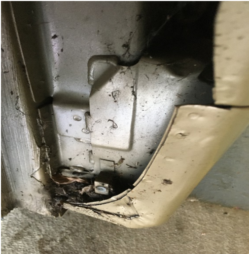
Mud trapped in inner wing.
